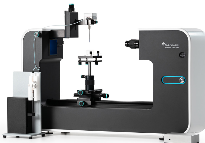
Figure 2. Theta Pulsating drop for interfacial rheology measurements
